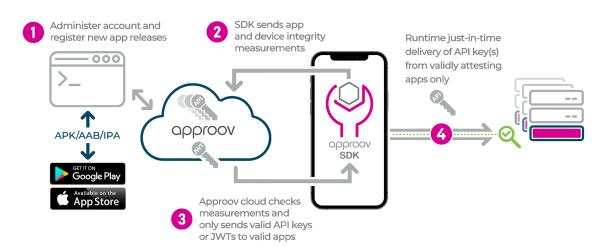
The diagram above illustrates the four-step flow of how Approov Runtime Secrets Protection works. This protection can be easily dropped into an existing app, that currently embeds API keys, with the minimum of changes: The steps are as follows:
