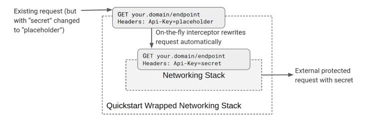
Integration is made as simple as possible by providing a networking stack that has exactly the same interface as the standard one, except that it provides runtime API key substitution.
